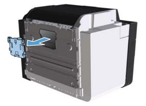
4. Insert the new separation pad, and screw it into place.
