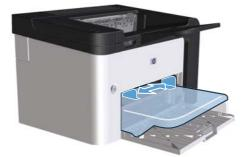
2. Place the media in the tray and adjust the media guides to the correct width.
