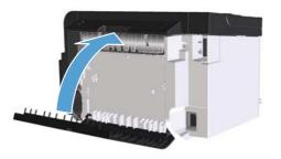
5. Reinstall the print cartridge and close the print-cartridge door.
